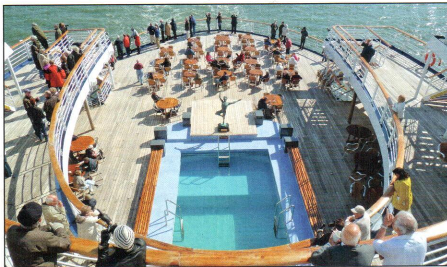
Tiered outdoor decks on the classic cruiser-spoon stern enhance the social interaction onboard.
